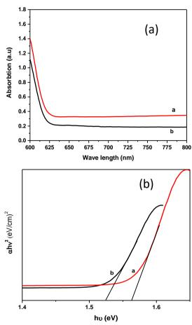
Fig: 4 a) UV-Vis absorption spectra and band gap of different reaction times of 3 hours and 6 hours as shown in fig.4 (a) & (b).
