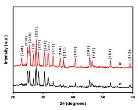
Fig.1 XRD pattern of the Bi<sub>2</sub>S<sub>3</sub> nanoparticles prepared with (a) 3 hours and (b) 6 hours.
