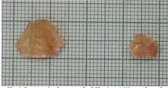
Fig.1 Grown single crystal of Glycine 4 Nitro-phenol
