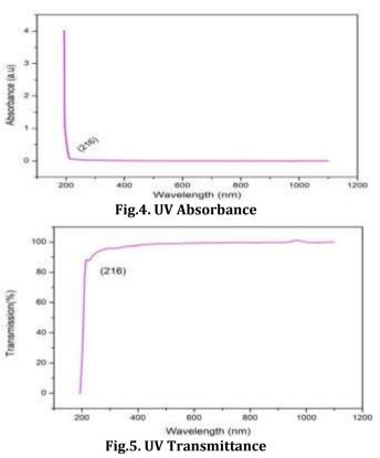
The transmittance graph is shown in Fig 5 and the transmittance is observed the cut off region is 216 nm and it is showing the good transmittance. Its resultant transmittance is maximum transmittance of glycine 4 Nitro-phenol crystal was used to nonlinear optical materials.
