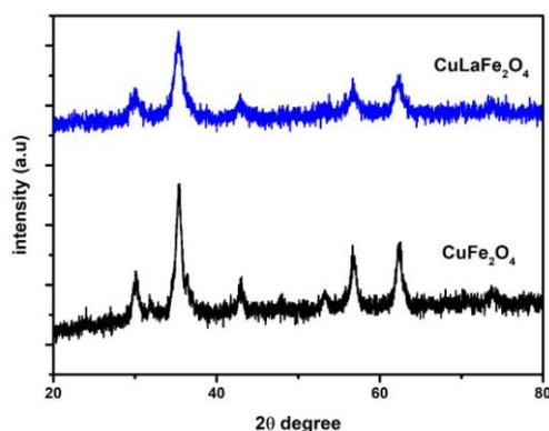
**Figure 1** X-ray Diffraction of CuLaFe $_2$ O $_4$  and CuFe $_2$ O $_4$
