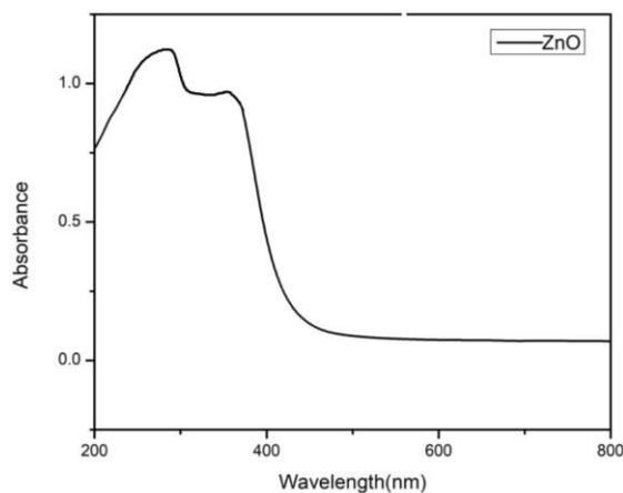
Fig 5. UV-Vis image of ZnO nanoparticles
