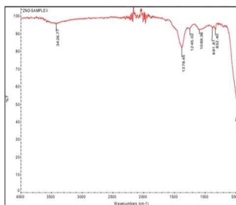
Fig 6. IR Spectrum of ZnO nanoparticles
