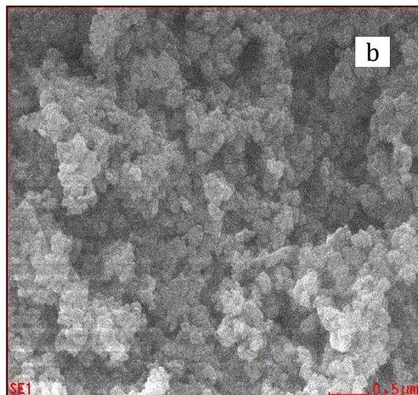
**Fig. 6. SEM image of MgO nanoparticles prepared in the presence of Orange Peel powder dried in a) Sun and b) Oven**
