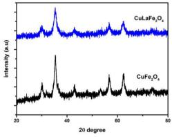
Figure 1X-ray Diffraction of CuLaFe<sub>2</sub>O<sub>4</sub> and CuFe<sub>2</sub>O<sub>4</sub>
