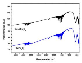
Figure 3 FTIR spectra of as-synthesised materials
