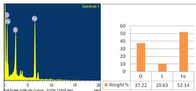
Fig.4. EDAX spectrum of Iron oxide nanoparticles
