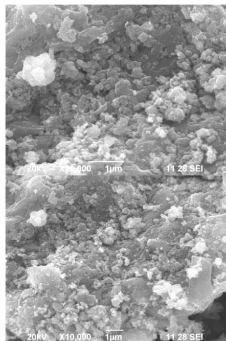
Fig.3. SEM micrograph of Iron oxide nanoparticles
