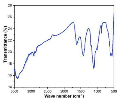
Fig.5. FTIR spectrum of Iron oxide nanoparticles
