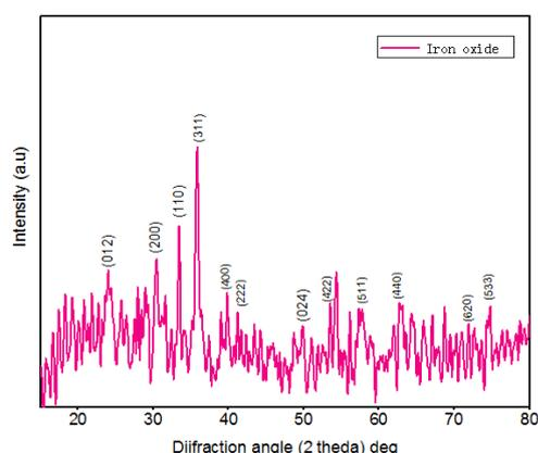
Fig.2. XRD pattern of Iron oxide nanoparticles
