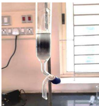
Figure 10. Ground water passed through bio-filter column.
